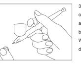
3.Color may often stick to the inside of Needle Cap and /or tip of Needle and Nozzle when an airbrush has been used for a long time. Wash off by a brush carefully not to damage Needle Tip.
