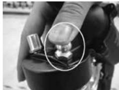
3. To avoid the risk of damage, the recommended working pressure / air source should not exceed 10.34 Bar (150psi).
