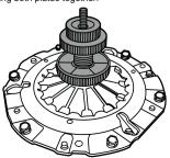
Turn both plates over. Slide the plates sideways until their edges become parallel.Tighten the conical wheel a bit further to keep both plates firm.
