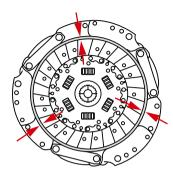
4. Install both plates on the flywheel, tightening their screws crosswise. Once the clutch assembly is complete, remove the tool by turning the conical and the small wheels counterclockwise.
