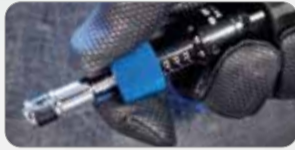
Set torque using the blue band
